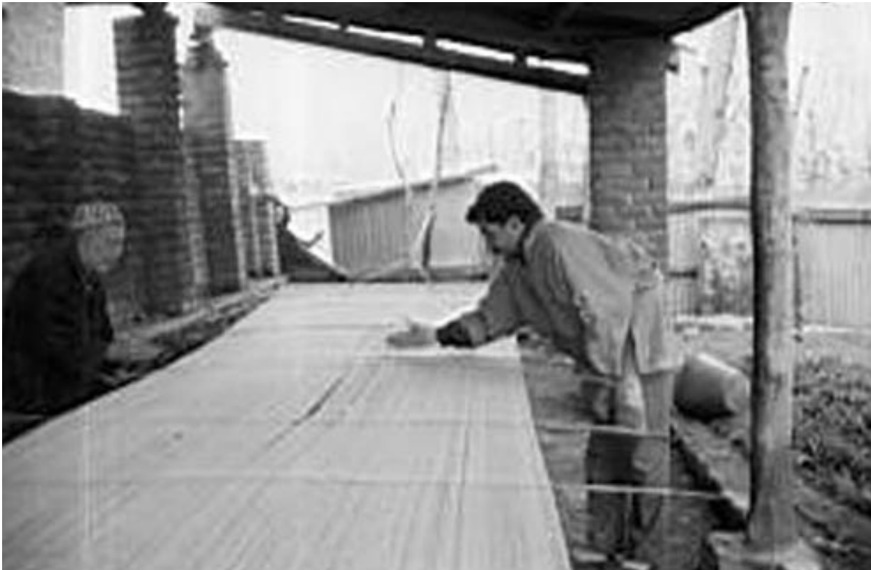
Preparing the warp for a shahtoosh shawl.
